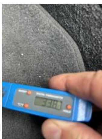
Temp Reading – Heaters on hot
