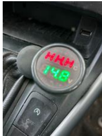
12V Battery Charging
