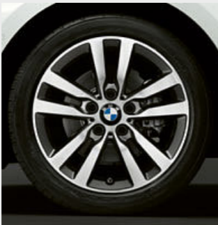
□ 17" light alloy Double-spoke style 655 wheels, 7.5J x 17 with 225/45 R17 tyres. (Optional for SE and Sport models).
