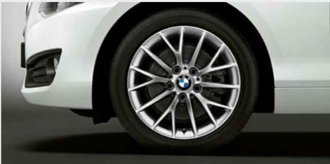
■ 17" light alloy Y-spoke style 380 wheels, Reflex Silver, 7J x 17 with 205/50 R17 tyres. (Standard for SE models).
