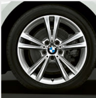
□ 18" light alloy Double-spoke style 385 wheels, front 7.5J x 18 with 225/40 R18, rear 8J x 18 with 245/35 R18 run-flat tyres. (Optional for SE and Sport models).
