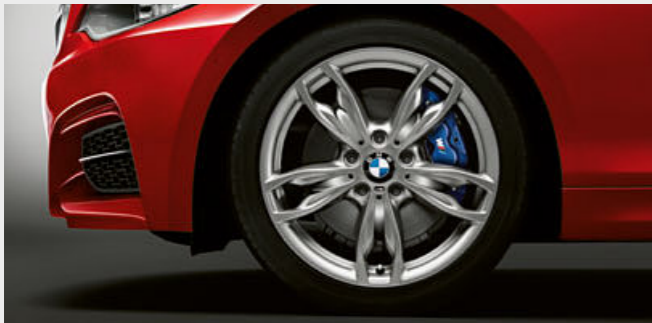
■ 18" M light alloy Double-spoke style 436 M wheels, Ferric Grey, front 7.5J x 18 with 225/40 R18, rear 8J x 18 with 245/35 R18 tyres. (Standard for M240i models).
